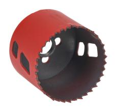
MK Morse hole saw, 2-1/2in (64mm), bi-metal cobalt, hardened steel backer, varied tooth, 1-15/16in (50mm) maximum cutting depth.
