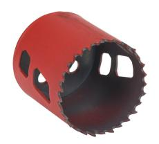
MK Morse hole saw, 2in (51mm), bi-metal cobalt, hardened steel backer, varied tooth, 1-15/16in (50mm) maximum cutting depth.
