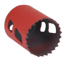
MK Morse hole saw, 1-3/4in (44mm), bi-metal cobalt, hardened steel backer, varied tooth, 1-15/16in (50mm) maximum cutting depth.
