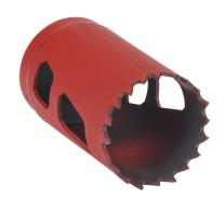
MK Morse hole saw, 1-3/8in (35mm), bi-metal cobalt, hardened steel backer, varied tooth, 1-15/16in (50mm) maximum cutting depth.
