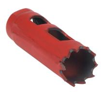
MK Morse hole saw, 3/4in (19mm), bi-metal cobalt, hardened steel backer, varied tooth, 1-15/16in (50mm) maximum cutting depth.
