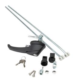
Hammond enclosure latch, combination keylocking/padlocking, 1/4-turn handle, 3-point, die-cast zinc, black matte finish. For use with less than 60in (H) NEMA 4 and NEMA 12 enclosures. (2) keys included.
