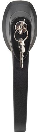
Hammond enclosure latch, combination keylocking/padlocking, 1/4-turn handle, 1-point, die-cast zinc, black matte finish. For use with single-door NEMA 4 and NEMA 12 enclosures. (2) keys included.
