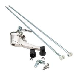
Hammond enclosure latch, padlocking with defeater, 1/4-turn handle, 3-point, 316 stainless steel. For use with less than 60in (H) NEMA 4X enclosures.
