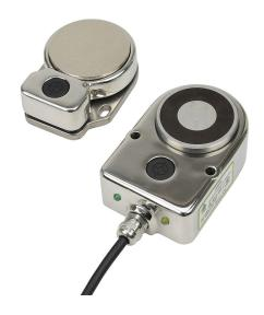
IDEM safety switch set, non-contact uniquely coded RFID, magnetic, 24 VDC to lock, 600N holding force, (4) N.O., (2) N.C. safety output(s), 316 stainless steel housing, 64 x 96 x 37mm, (1) 8-pin M12 quick-disconnect, 9.8in/250mm cable length.
