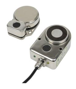
IDEM safety switch set, non-contact uniquely coded RFID, magnetic, 24 VDC to lock, 600N holding force, (2) N.C. safety output(s), 316 stainless steel housing, 64 x 96 x 37mm, pigtail, 16.4ft/5m cable length.
