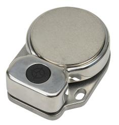
IDEM safety switch actuator, replacement, non-contact master coded RFID, 600N holding force, 316 stainless steel housing, 64 x 88 x 30mm.
