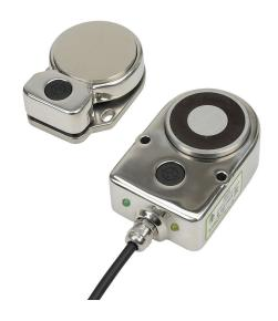
IDEM safety switch set, non-contact master coded RFID, magnetic, 24 VDC to lock, 600N holding force, (2) N.C. safety output(s), 316 stainless steel housing, 64 x 96 x 37mm, (1) 8-pin M12 quick-disconnect, 9.8in/250mm cable length.
