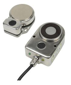
IDEM safety switch set, non-contact master coded RFID, magnetic, 24 VDC to lock, 600N holding force, (2) N.C. safety output(s), 316 stainless steel housing, 64 x 96 x 37mm, pigtail, 16.4ft/5m cable length.
