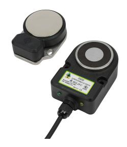
IDEM safety switch set, non-contact uniquely coded RFID, magnetic, 24 VDC to lock, 1000N holding force, (2) N.C. safety output(s), plastic housing, 64 x 96 x 37mm, (1) 8-pin M12 quick-disconnect, 9.8in/250mm cable length.
