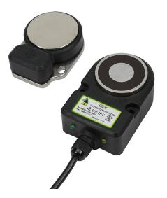
IDEM safety switch set, non-contact uniquely coded RFID, magnetic, 24 VDC to lock, 1000N holding force, (2) N.C. safety output(s), plastic housing, 64 x 96 x 37mm, pigtail, 16.4ft/5m cable length.
