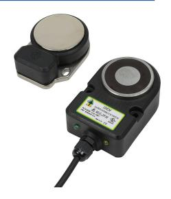
IDEM safety switch set, non-contact master coded RFID, magnetic, 24 VDC to lock, 1000N holding force, (2) N.C. safety output(s), plastic housing, 64 x 96 x 37mm, (1) 8-pin M12 quick-disconnect, 9.8in/250mm cable length.
