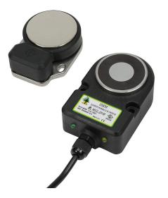
IDEM safety switch set, non-contact master coded RFID, magnetic, 24 VDC to lock, 1000N holding force, (2) N.C. safety output(s), plastic housing, 64 x 96 x 37mm, pigtail, 16.4ft/5m cable length.
