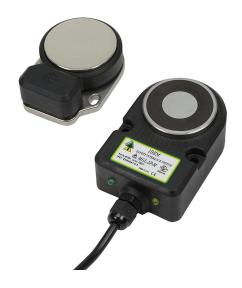
IDEM safety switch set, non-contact master coded RFID, magnetic, 24 VDC to lock, 1000N holding force, (2) N.C. safety output(s), plastic housing,  $64 \times 96 \times 37$ mm, pigtail, 16.4ft/5m cable length.
