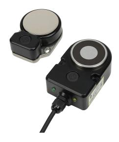
IDEM safety switch set, non-contact uniquely coded RFID, magnetic, 24 VDC to lock, 1000N holding force, (2) N.C. safety output(s), die-cast aluminum housing, 64 x 96 x 37mm, (1) 8-pin M12 quick-disconnect, 9.8in/250mm cable length.
