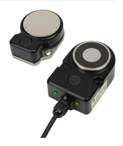
IDEM safety switch set, non-contact uniquely coded RFID, magnetic, 24 VDC to lock, 1000N holding force, (2) N.C. safety output(s), die-cast aluminum housing, 64 x 96 x 37mm, (1) 8-pin M12 quick-disconnect, 9.8in/250mm cable length.
