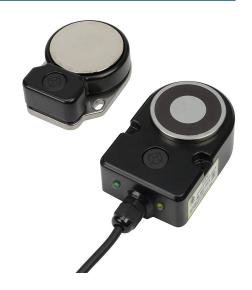
IDEM safety switch set, non-contact master coded RFID, magnetic, 24 VDC to lock, 1000N holding force, (2) N.C. safety output(s), die-cast aluminum housing, 64 x 96 x 37mm, (1) 8-pin M12 quick-disconnect, 9.8in/250mm cable length.
