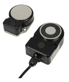
IDEM safety switch set, non-contact master coded RFID, magnetic, 24 VDC to lock, 1000N holding force, (2) N.C. safety output(s), die-cast aluminum housing, 64 x 96 x 37mm, pigtail, 16.4ft/5m cable length.
