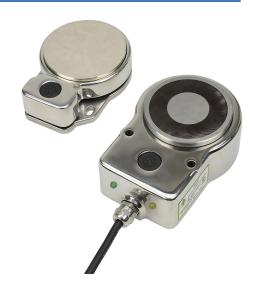
IDEM safety switch set, non-contact uniquely coded RFID, magnetic, 24 VDC to lock, 1200N holding force, (2) N.C. safety output(s), 316 stainless steel housing, 80 x 115 x 43mm, (1) 8-pin M12 quick-disconnect, 9.8in/250mm cable length.
