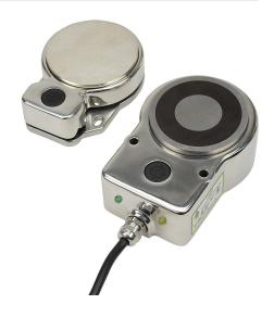
IDEM safety switch set, non-contact uniquely coded RFID, magnetic, 24 VDC to lock, 1200N holding force, (2) N.C. safety output(s), 316 stainless steel housing, 80 x 115 x 43mm, pigtail, 16.4ft/5m cable length.
