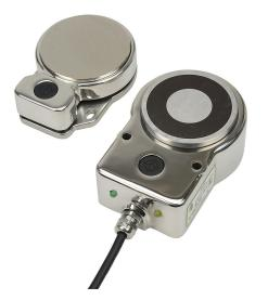
IDEM safety switch set, non-contact master coded RFID, magnetic, 24 VDC to lock, 1200N holding force, (2) N.C. safety output(s), 316 stainless steel housing, 80 x 115 x 43mm, (1) 8-pin M12 quick-disconnect, 9.8in/250mm cable length.
