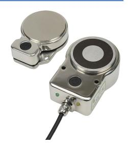
IDEM safety switch set, non-contact master coded RFID, magnetic, 24 VDC to lock, 1200N holding force, (2) N.C. safety output(s), 316 stainless steel housing, 80 x 115 x 43mm, (1) 8-pin M12 quick-disconnect, 9.8in/250mm cable length.
