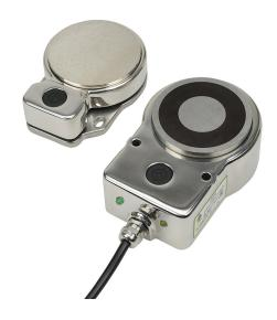
IDEM safety switch set, non-contact master coded RFID, magnetic, 24 VDC to lock, 1200N holding force, (2) N.C. safety output(s), 316 stainless steel housing, 80 x 115 x 43mm, pigtail, 16.4ft/5m cable length.
