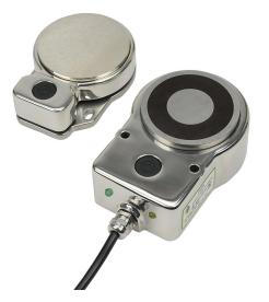
IDEM safety switch set, non-contact master coded RFID, magnetic, 24 VDC to lock, 1200N holding force, (2) N.C. safety output(s), 316 stainless steel housing, 80 x 115 x 43mm, pigtail, 16.4ft/5m cable length.
