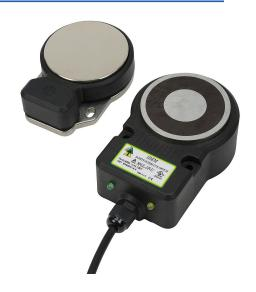
IDEM safety switch set, non-contact uniquely coded RFID, magnetic, 24 VDC to lock, 1500N holding force, (2) N.C. safety output(s), plastic housing, 80 x 115 x 43mm, (1) 8-pin M12 quick-disconnect, 9.8in/250mm cable length.
