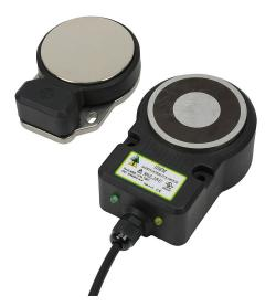
IDEM safety switch set, non-contact uniquely coded RFID, magnetic, 24 VDC to lock, 1500N holding force, (2) N.C. safety output(s), plastic housing, 80 x 115 x 43mm, (1) 8-pin M12 quick-disconnect, 9.8in/250mm cable length.
