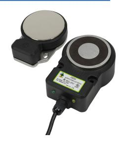
IDEM safety switch set, non-contact uniquely coded RFID, magnetic, 24 VDC to lock, 1500N holding force, (2) N.C. safety output(s), plastic housing, 80 x 115 x 43mm, pigtail, 16.4ft/5m cable length.
