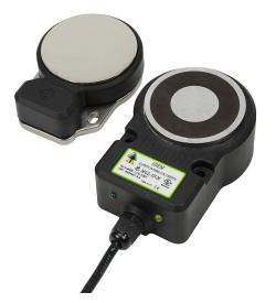
IDEM safety switch set, non-contact master coded RFID, magnetic, 24 VDC to lock, 1500N holding force, (2) N.C. safety output(s), plastic housing, 80 x 115 x 43mm, (1) 8-pin M12 quick-disconnect, 9.8in/250mm cable length.
