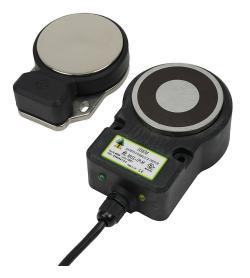
IDEM safety switch set, non-contact master coded RFID, magnetic, 24 VDC to lock, 1500N holding force, (2) N.C. safety output(s), plastic housing, 80 x 115 x 43mm, pigtail, 16.4ft/5m cable length.
