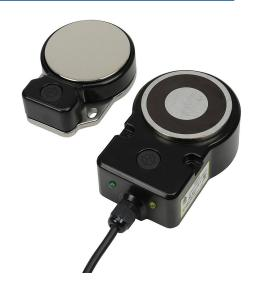
IDEM safety switch set, non-contact uniquely coded RFID, magnetic, 24 VDC to lock, 1500N holding force, (2) N.C. safety output(s), die-cast aluminum housing, 80 x 115 x 43mm, pigtail, 16.4ft/5m cable length.
