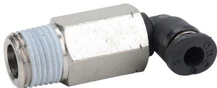
NITRA pneumatic push-to-connect fitting, long elbow, rotating, thermoplastic (PBT) body, nickel-plated brass threads, thread sealant, (1) 1/8in male NPT to (1) 1/8in push-to-connect. Package of 5.
