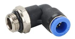
NITRA pneumatic push-to-connect fitting, elbow, rotating, thermoplastic (PBT) body, nickel-plated brass threads, thread sealant, (1) G1/4 male BSPP to (1) 5/16in (8mm) push-to-connect. Package of 5.
