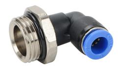
NITRA pneumatic push-to-connect fitting, elbow, rotating, thermoplastic (PBT) body, nickel-plated brass threads, thread sealant, (1) G1/2 male BSPP to (1) 5/16in (8mm) push-to-connect. Package of 5.
