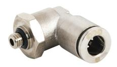
NITRA pneumatic push-to-connect fitting, elbow, rotating, nickel-plated brass body, nickel-plated brass threads, (1) M5 x 0.8 male ISO to (1) 6mm push-to-connect. Package of 5.
