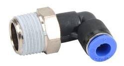
NITRA pneumatic push-to-connect fitting, elbow, rotating, thermoplastic (PBT) body, nickel-plated brass threads, thread sealant, (1) R3/8 male BSPT to (1) 6mm push-to-connect. Package of 5
