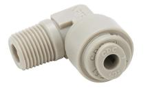
HydroMode potable water push-to-connect fitting, male, elbow, acetal body, acetal threads, (1) 5/32in tube to (1) 1/8in male NPT connection(s), NSF/ANSI 61. Package of 5.
