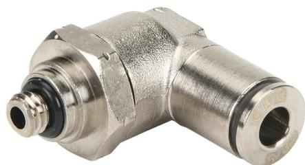
NITRA pneumatic push-to-connect fitting, elbow, rotating, nickel-plated brass body, nickel-plated brass threads, (1) #10-32 male UNF to (1) 5/32in (4mm) push-to-connect. Package of 5.
