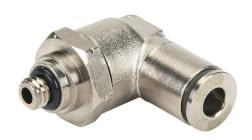
NITRA pneumatic push-to-connect fitting, male, elbow, rotating, nickel-plated brass body, nickel-plated brass threads, 5/32in (4mm) push-to-connect to #10-32 threaded. Package of 5.
