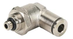
NITRA pneumatic push-to-connect fitting, elbow, rotating, nickelplated brass body, nickel-plated brass threads, (1) #10-32 male UNF to (1) 5/32in (4mm) push-to-connect. Package of 5.
