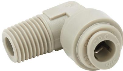
HydroMode potable water push-to-connect fitting, male, elbow, acetal body, acetal threads, (1) 5/16in tube to (1) 1/4in male NPT connection(s), NSF/ANSI 61. Package of 5.
