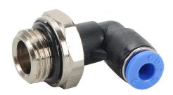
NITRA pneumatic push-to-connect fitting, elbow, rotating, thermoplastic (PBT) body, nickel-plated brass threads, thread sealant, (1) G1/4 male BSPP to (1) 5/32in (4mm) push-to-connect. Package of 5.
