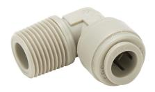
HydroMode potable water push-to-connect fitting, male, elbow, acetal body, acetal threads, (1) 3/8in tube to (1) 3/8in male NPT connection(s), NSF/ANSI 61. Package of 5.
