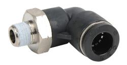
NITRA pneumatic push-to-connect fitting, elbow, rotating, thermoplastic (PBT) body, nickel-plated brass threads, thread sealant, (1) 1/8in male NPT to (1) 3/8in push-to-connect. Package of 5.
