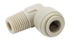
HydroMode potable water push-to-connect fitting, male, elbow, acetal body, acetal threads, (1) 3/8in tube to (1) 1/4in male NPT connection(s), NSF/ANSI 61. Package of 5.
