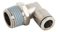
NITRA pneumatic push-to-connect fitting, elbow, rotating, nickelplated brass body, nickel-plated brass threads, thread sealant, (1) 1/2in male NPT to (1) 3/8in push-to-connect. Package of 5.
