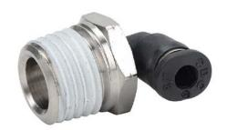
NITRA pneumatic push-to-connect fitting, male, elbow, rotating, thermoplastic (PBT) body, nickel-plated brass threads, 1/8in tube to 1/4in NPT connection(s). Package of 5.
