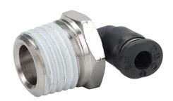
NITRA pneumatic push-to-connect fitting, elbow, rotating, thermoplastic (PBT) body, nickel-plated brass threads, thread sealant, (1) 1/4in male NPT to (1) 1/8in push-to-connect. Package of 5.
