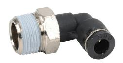
NITRA pneumatic push-to-connect fitting, elbow, rotating, thermoplastic (PBT) body, nickel-plated brass threads, thread sealant, (1) R3/8 male BSPT to (1) 1/4in push-to-connect. Package of 5.
