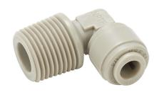
HydroMode potable water push-to-connect fitting, male, elbow, acetal body, acetal threads, (1) 1/4in tube to (1) 3/8in male NPT connection(s), NSF/ANSI 61. Package of 5.
