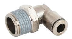
NITRA pneumatic push-to-connect fitting, elbow, rotating, nickel-plated brass body, nickel-plated brass threads, thread sealant, (1) R3/8 male BSPT to (1) 1/4in push-to-connect. Package of 5.
