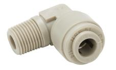
HydroMode potable water push-to-connect fitting, male, elbow, acetal body, acetal threads, (1) 1/4in tube to (1) 1/8in male NPT connection(s), NSF/ANSI 61. Package of 5.
