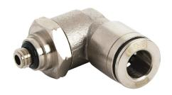
NITRA pneumatic push-to-connect fitting, elbow, rotating, nickel-plated brass body, nickel-plated brass threads, (1) #10-32 male UNF to (1) 1/4in push-to-connect. Package of 5.
