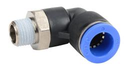
NITRA pneumatic push-to-connect fitting, elbow, rotating, thermoplastic (PBT) body, nickel-plated brass threads, thread sealant, (1) R1/4 male BSPT to (1) 12mm push-to-connect. Package of 5.
