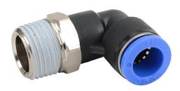
NITRA pneumatic push-to-connect fitting, elbow, rotating, thermoplastic (PBT) body, nickel-plated brass threads, thread sealant, (1) R1/2 male BSPT to (1) 12mm push-to-connect. Package of 5.
